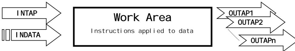
The essential difference between the input and insert streams is that each record in the input stream generates a single logical record, or case in the work area, whereas the records in the insert stream are treated as separate elements of a logical record identified by a case ID.
